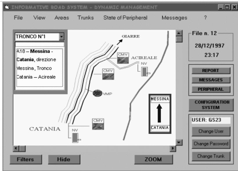
Fig. 10 - Detailed graphic representation concerning the Catania-Acireale Section (Highway A18 Messina-Catania, direction Messina). The locations of different peripherals are particularly evidenced.
