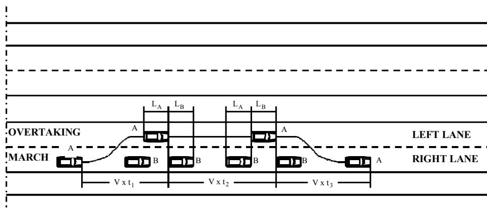
Fig. 2 - Scheme of highway overtaking.
