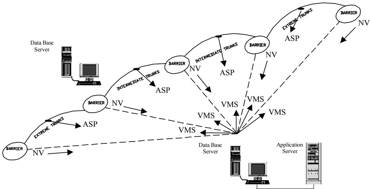
Fig. 7 - Architecture of the Information System for the dynamic management of road serviceability.
