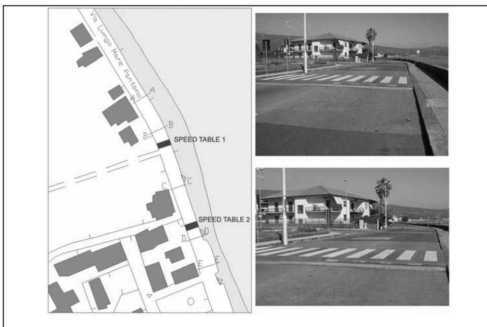
**Figure 2 Speed tables in Lungo Mare Pantano street (Riposto)**
