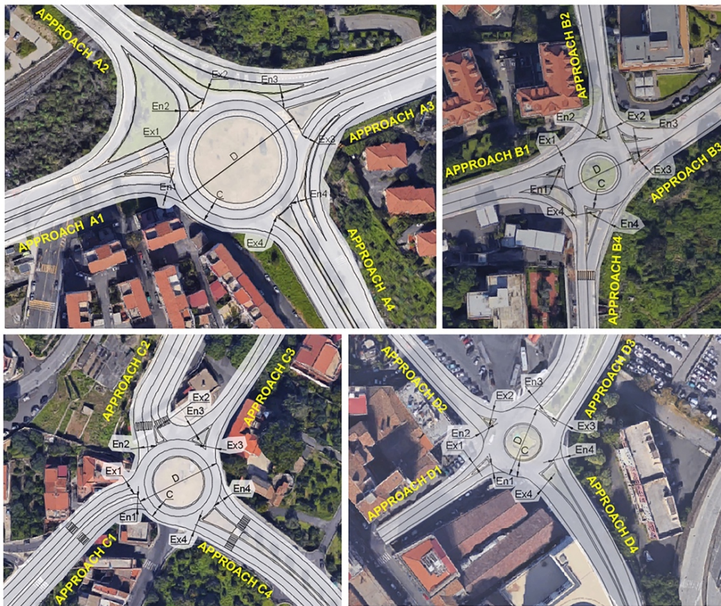
Figure 2: Geometric plan views of the four roundabouts studied
