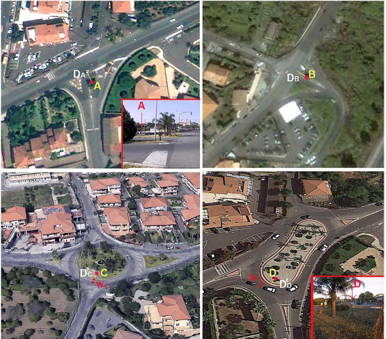
Fig. 2—Arrangement of sound level meters at standard intersections and roundabouts: reference distances for measurements (DA, DB, D'C, D'D, WC, WD).
